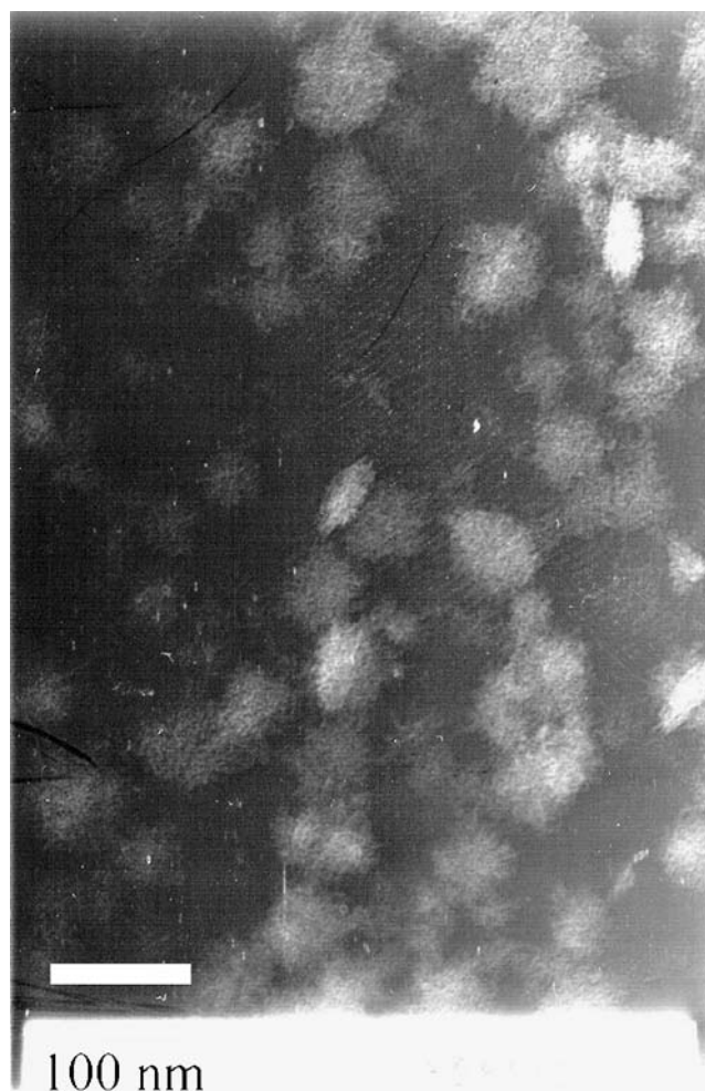
Fig. 1 Transmission electron microscopy image for a sample dried from a \text{ZrO}_2 aqueous suspension
